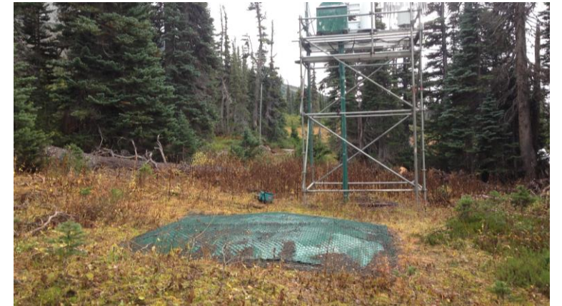
Snow pillow and meteorological station in October
